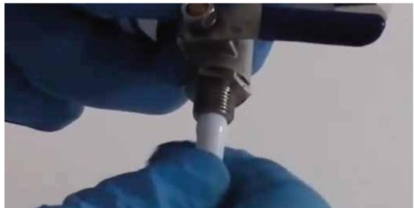
Push the tubing onto the stem of the ball valve. Ensure it has been pushed all the way over the little ridge.
