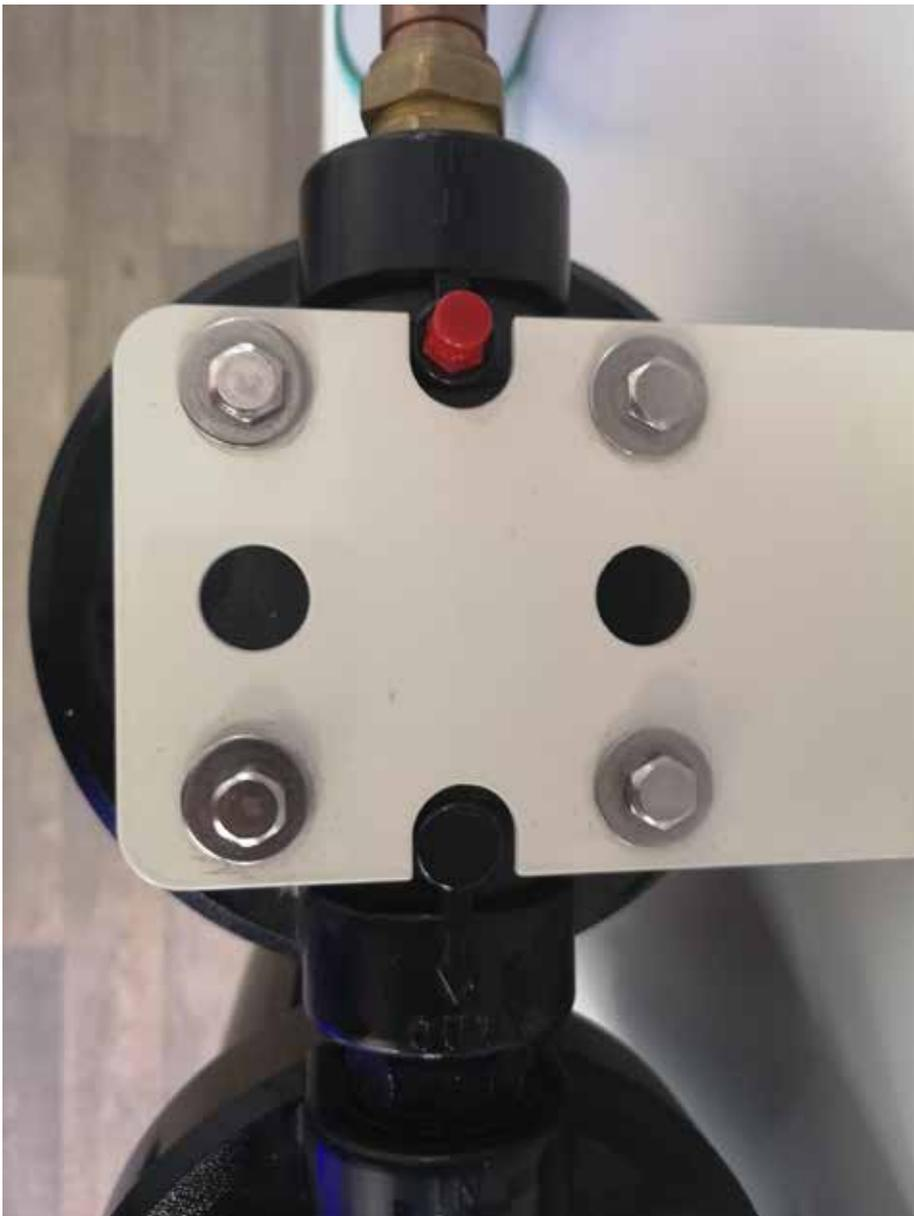
Use the screws provided with your filter housing to mount the bracket to the head of the filter unit. The screws are self-tapping and will thread themselves into the sockets of the housing head. Use a spanner or socket spanner for this.
