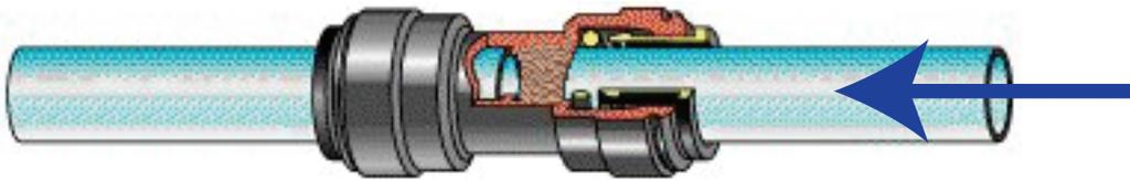
**Step 4:** Now push the tubing into the fitting harder until the tube stop is felt. The collet has stainless steel teeth which hold the tubing in position while the O-ring provides a permanent leak proof seal.
