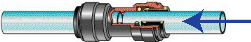
**Step 5:** Pull on the tubing away from the fitting and make sure it stays firmly in place. It is good practice to test the connection with pressurized water before finishing installation.
