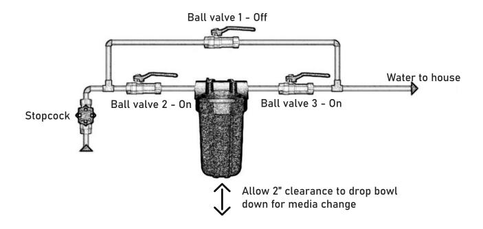
Ensure the MaxiSOFT is mounted on horizontal pipework with the media bowl positioned vertically with 2" clearance for the bowl to be dropped when replacing the media.
